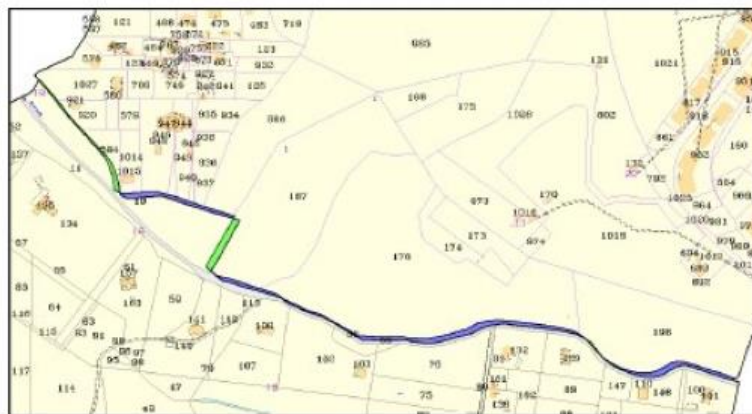
2 Overlapping of the vector map files on the original maps before the topological consistency recovery
