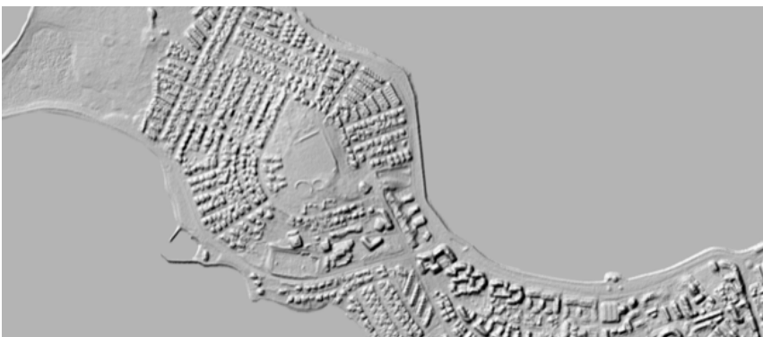
Figure 2 Mosaic, using a median value of all possible DEMs at each cell location
