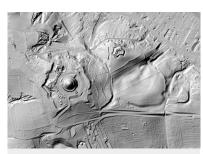
Example of analytical shading in DTM visualisation
