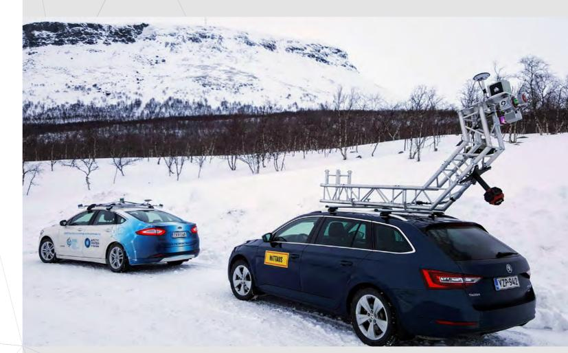
The NLS Finland own-built autonomous car is seen here on the left with the high-definition mapping car on the right.
