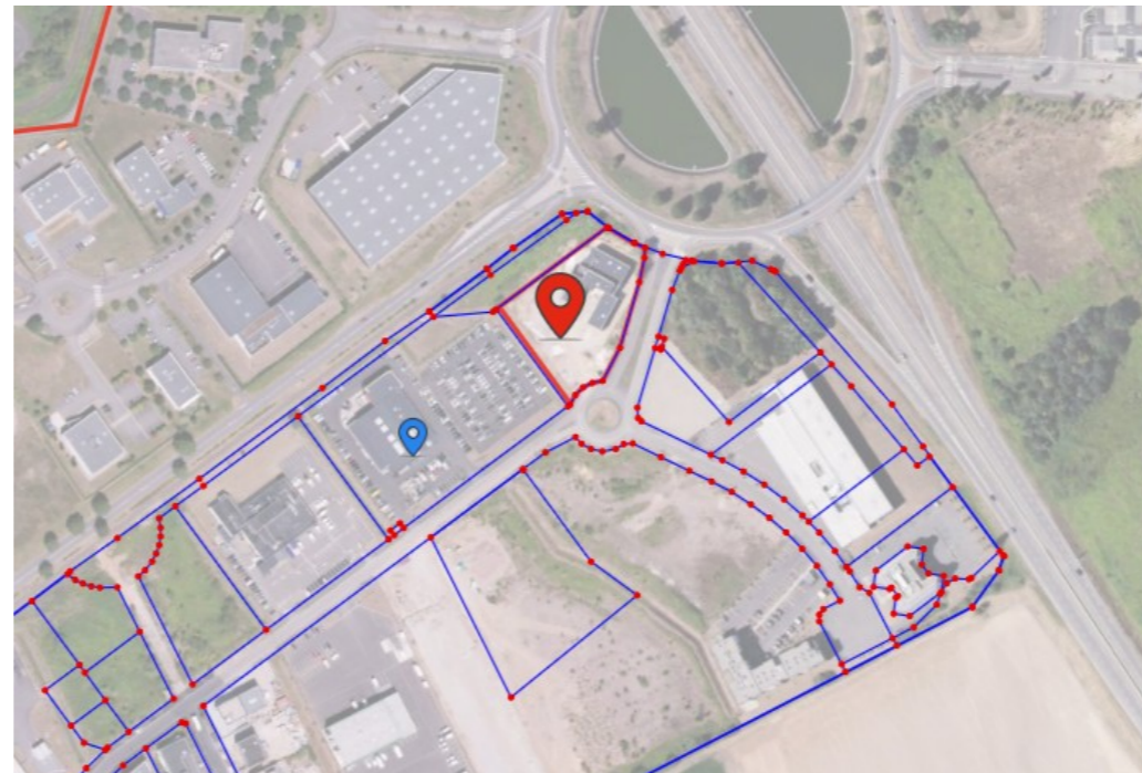
direct use of CAD data of the land surveyors (screenshot of the "Geofoncier" platform)
