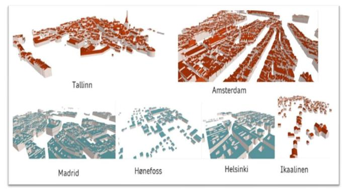
Example of the GEOE3 data integration platform. Buildings in red are at Level of Detail 2 (LoD2) and buildings in blue are at Level of Detail 1 (LoD1). LoD1 is generated on the fly using the height of the building (Spain) or the digital surface model (Finland, Norway).
