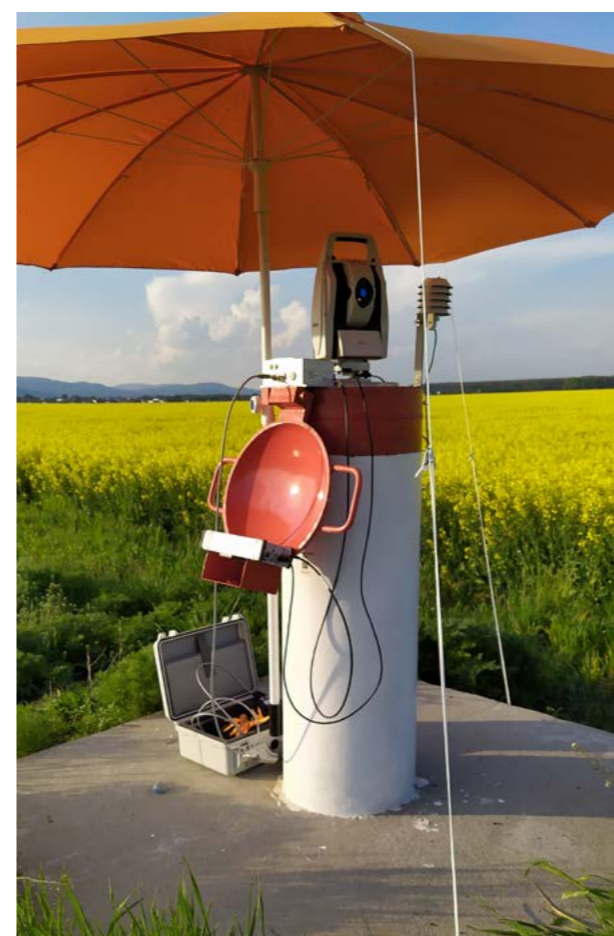
EDM instrument prepared for testing
