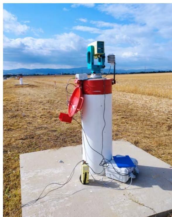
Reference measurement of the calibration baseline
