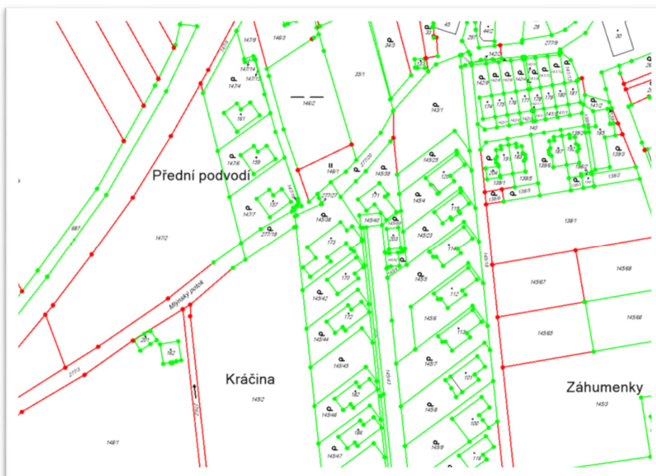
Figure 15: Digital Cadastral Map from Czech Republic with indication of refined and agreed boundaries (green) and less accurate non-agreed boundaries (green).
