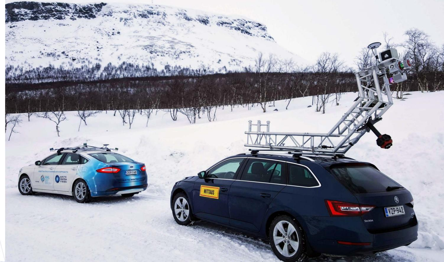
The NLS Finland own-built autonomous car is seen here on the left with the high-definition mapping car on the right.
